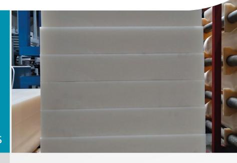
Especially for the production of special machined parts, AGRU can now manufacture blocks with a thickness of up to 120 mm in addition to solid bars and press sheets. Usually, thick components are manufactured in one pressing process, but the new AGRU blocks are produced in a continuous extrusion process. The typical applications of thick blocks are mainly in the mechanical production of special parts, which are used in industry and in container, apparatus and pipeline construction.
